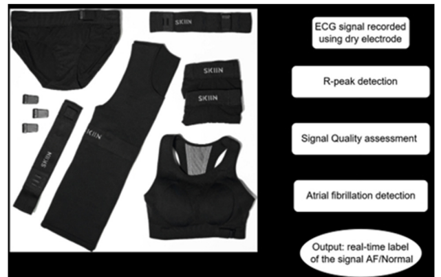
Figure1: Device providing textile ECG and structure of the proposed AF detection method
